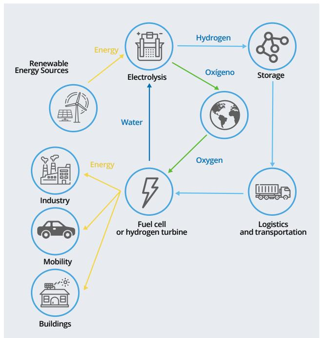
An electrolyser is an electrochemical device where water molecule is split into hydrogen and oxygen. Oxygen is vented and hydrogen stored on tanks or vessels. A fuel cell in a device with the opposite function, it is fed with hydrogen from tanks, takes oxygen from air and delivers electrical power and water. Alternatively and depending on the volume of hydrogen available, turbines can be used to convert hydrogen into electricity (see section 1.6).
